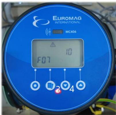
Use button #3 or 4 to adjust this value. At 10, this meter will send 1 pulse for every 10 units that pass through the sensor.
