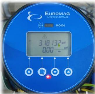
STEP 1- Press any button to wake up Red LED
