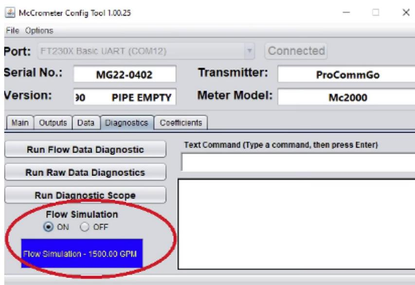
To turn off flow simulation simply click the "OFF" bubble.
