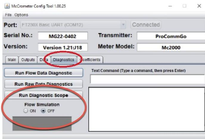
You will be prompted to enter the flow you wish to simulate (Note: flow will be displayed in gallons per minute). A blue box will confirm your flow simulation is running. Verify the same rate is displayed on your meters' display.
