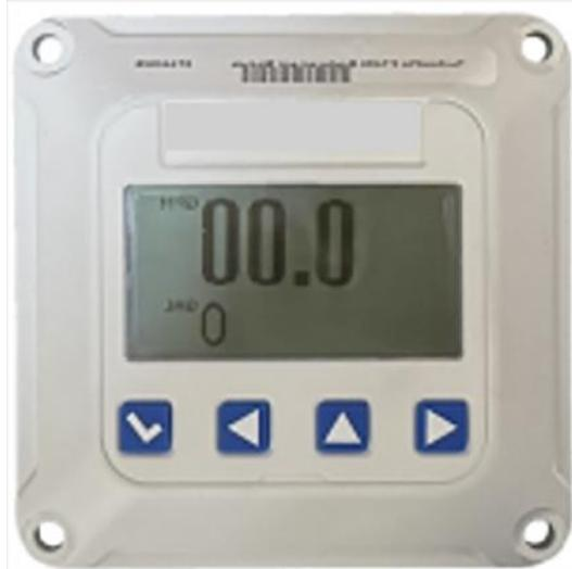
These units calculate rate and total using a K-factor input. Click any button to bring you to the first menu screen. The first tab is SETK (K-factor.) Press the check mark  to enter the SETK tab. The K-factor must be entered as pulses per GALLON. And use the check mark to exit the SETK tab. The PS32 and the PM04 units will have the K-factor preloaded and locked out.
