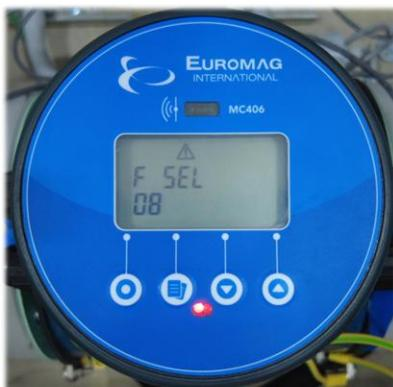
Use button #4 to navigate to **(Pulse Technical Unit Settings)**
