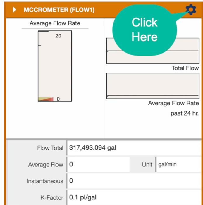
4. Click on General and you'll see all your configuration parameters to define your Flow K-Factor, Flow Total, Flow Rate units and time base. Here you can also set your flow total to match your meter when configuring on a meter that has been in service.
