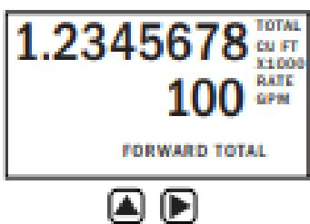
Once you have adjusted or confirmed the SET P, use the hold and tap procedure (cover the UP arrow and while continuing to cover the UP arrow, tap and release the RIGHT arrow) to get back to the first menu screen. RIGHT arrow to the EXIT tab and use the hold and tap procedure again to return to the home screen.
