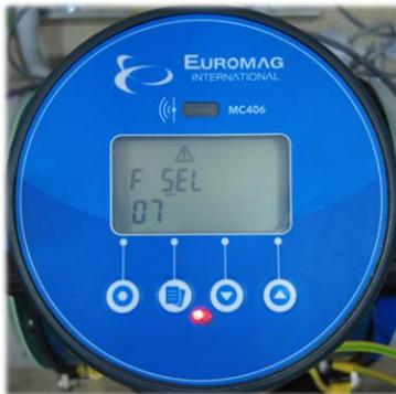
Use button #4 to navigate to **(Pulse Volume Setting)**
