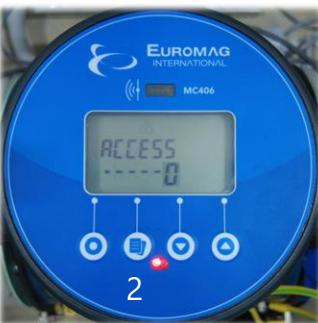
STEP 3- Press #2 button to 6 times to move cursor and enter Function Menu.
