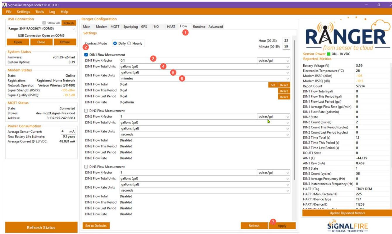
The process for calculating the K-Factor and the results are the same as doing this with the SignalFire Cloud. It's recommended to be connected to the RANGER when configuring these parameters.
