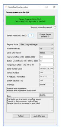
**Sensor Modbus ID:** To change the Sensor Modbus ID, type a number between 1 and 31. If it is different than the current Sensor Modbus ID, the button to *Change Sensor Modbus ID* will be enabled. Clicking it will change both the Sensor Modbus ID and the Sentinel Modbus ID.
