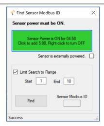
If the Sensor Modbus ID is found but does not match the Sentinel Modbus ID, click **Yes** in the pop-up message box to change the Sentinel Modbus ID.
