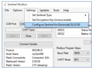
The Electrolab DLS2100 is now fully configured for wireless communication. When using **SignalFire ToolKit v2.2.34.00 or higher**, the program steps are set based on the register mode configured in the Electrolab. Otherwise, the program steps assume the default register mode of 16-bit unsigned integers. To set the register mode, see section Configure Electrolab Settings.
