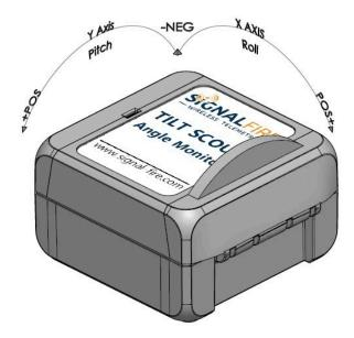
Note that the X and Y angles reported by the device are parallel to the X and Y axis of the enclosure.
