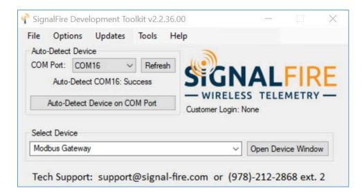
Select the COM port associated with the Tilt Scout and click "Auto-Detect Device on COM Port." This will open the device configuration window, where all device settings can be configured.
