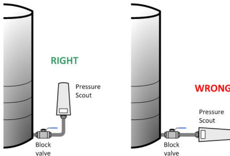
How you install the Pressure Scout may also depend on the process fluid. Refer to the diagram below for installation on gas, steam, or liquid.
