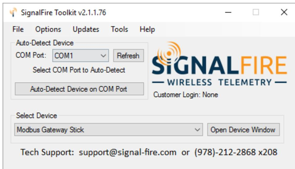
Select the COM port associated with the Pressure Scout and click "Auto-Detect Device on COM Port." This will open the device configuration window, where all device settings can be configured.
