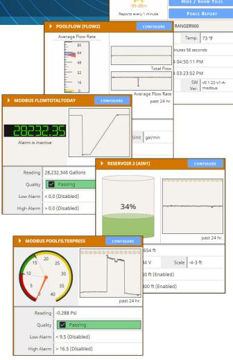
Tile View for measurements with customizable widgets
