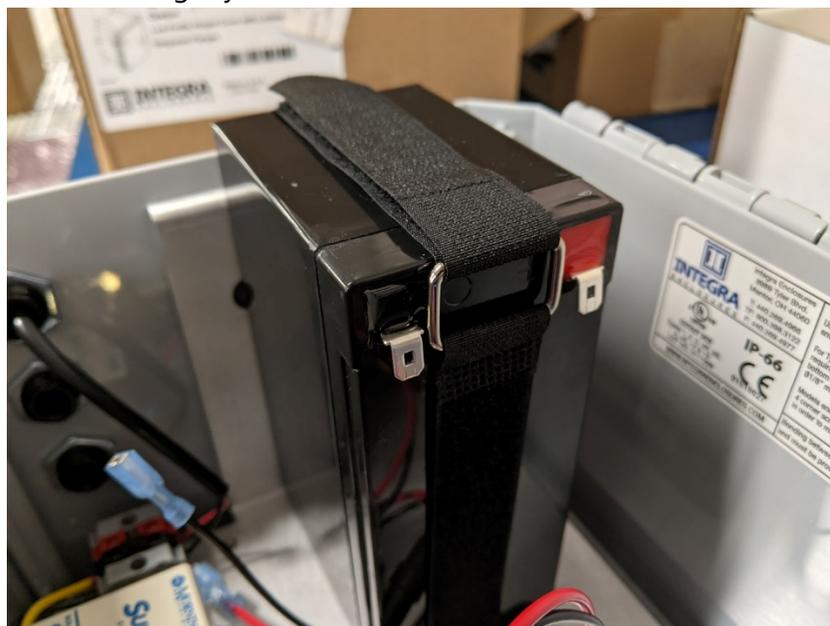
5. Insert the disconnects on to the battery's tabs, red to red, black to black. The system will then be fully powered on.
