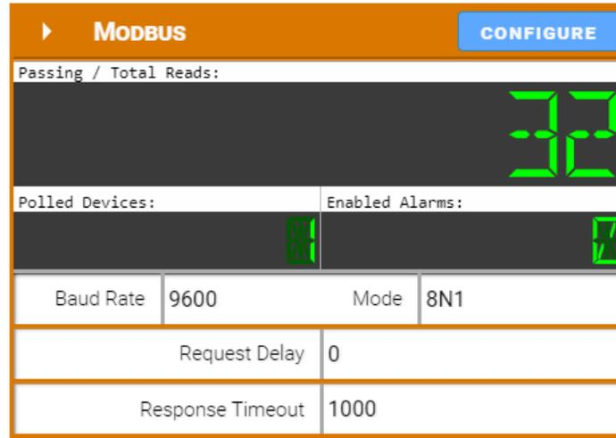
The Ranger can read up to 32 datapoints from up to 8 connected devices. To add a new register read, click on the '+' button. Each line needs to be specified with a Tag Name, and point to a Modbus Slave ID, register address, register data type, and read/write access. The register can also be tagged with units if needed. Click Apply to send the changes to the Ranger.
