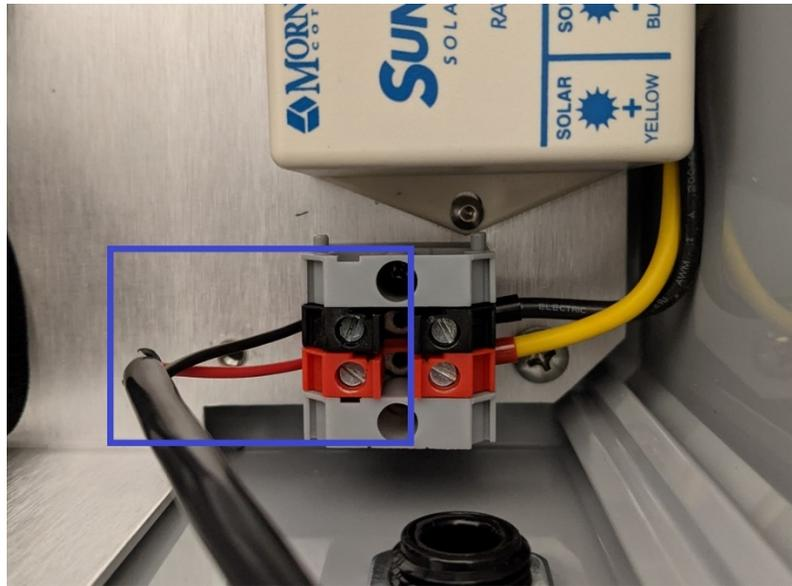
3. Tighten the cable gland until the solar panel cable is secure.
