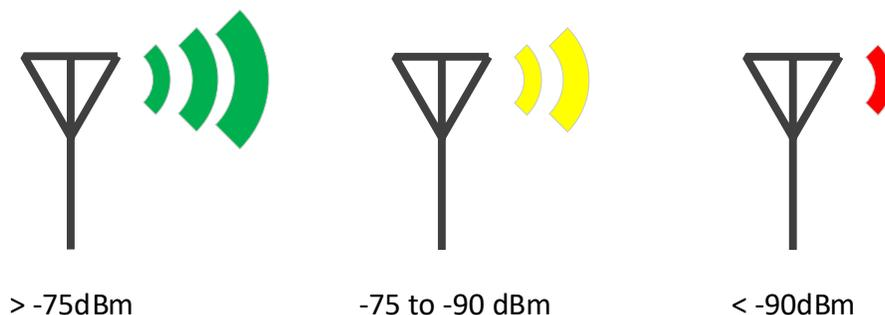
**To monitor the RSSI of any node, read register 65531 from that device's slave ID.** Seeing a node's RSSI jump around a wide range, or frequently hit below -100dBm may indicate installation issues, while seeing consistently good RSSIs but frequent missed check ins may indicate interference.
