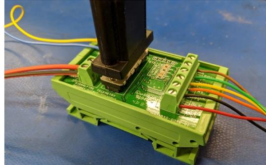
Accessible on the SignalFire website after registering for an account, this user-friendly PC application provides users with an interface to set a device's parameters, read their Modbus registers, and connect them to their network. The configuration cable converts from a user's computer USB to either a Serial DB-9 (typically for Gateway devices) or Serial 4-Pin (typically for node devices).
