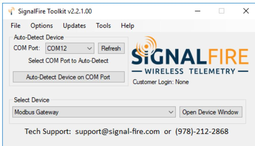
Screen image 1: After connecting the USB Serial cable to the Gateway or the USB 4 Pin cable to the node, click Autodetect on the main page of the SignalFire Toolkit to get started.
