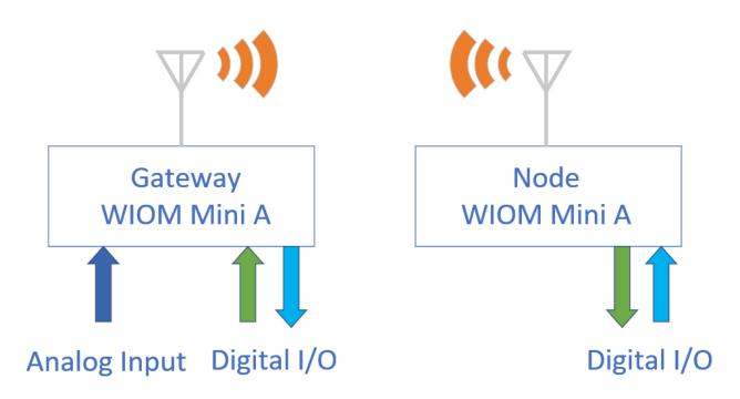
Point-to-Point Mode. Inputs from one module are mirrored as outputs on the other
