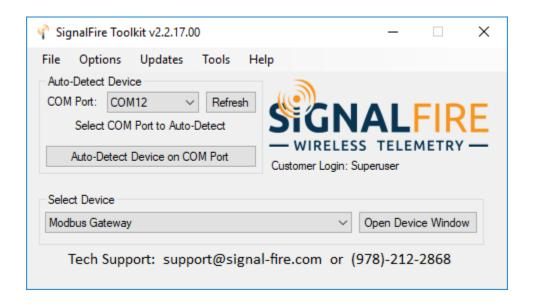
Select the COM port associated with the Wireless IO Module Mini and click "Auto-Detect Device on COM Port." This will open the device configuration window, where all device settings can be configured.
