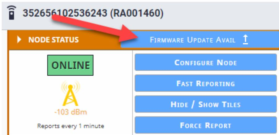
The screenshot shows a node status tile for a Ranger with ID 352656102536243 (RA001460). The tile is titled "NODE STATUS" and includes a "FIRMWARE UPDATE AVAIL" button with an upward arrow icon. A red arrow points to this button. Other elements include an "ONLINE" status, a signal strength indicator of -103 dBm, and a "Reports every 1 minute" note. On the right side, there are four blue buttons: "CONFIGURE NODE", "FAST REPORTING", "HIDE / SHOW TILES", and "FORCE REPORT".
