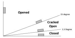
• Angle Mode: The device reports the average, minimum and maximum X and Y axis angles over the reporting interval along with a data distinguishing sequence number.
