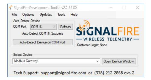
Select the COM port associated with the Tilt Scout and click "Auto-Detect Device on COM Port." This will open the device configuration window, where all device settings can be configured.
