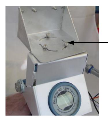
3 #8 Nuts and Flat Washers Align so the solar panel faces south (into the sun).
