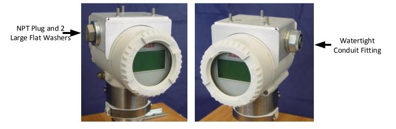
Note – Use Teflon tape on the threads on both fittings.
