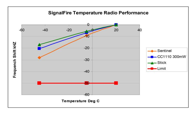
Note – You can see that the frequency shift is less than the limit. Also, if all the units are similar temperature, only the *frequency difference* matters, so that is much smaller.
