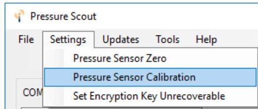
Calibration should be done with pressure applied to the Pressure Scout sensor. First, tie the sensor thread on the bottom to a pressure calibrator, or a line with a known stable pressure. Ideally, this pressure should be half the sensor span. For a 0-1,000PSI range Pressure Scout, for example, apply a stable 500PSI to the sensor.
