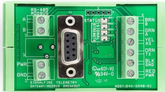
The breakout board above is included with the standard Modbus Stick and provides for easy wiring and a DIN rail mount. **PWR** and **GND** can be wired in to the breakout board, as well as RS485 A/B.
