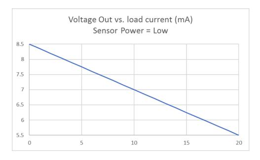
If the Sentinel-Solar is used the maximum load current is limited to 14mA.
