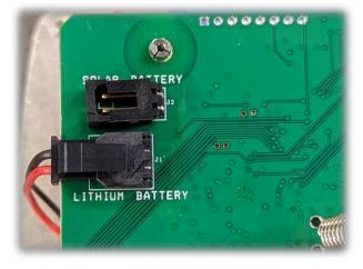
Only connect either the Lithium batter OR the Solay battery. **Never connect both at the same time.**
