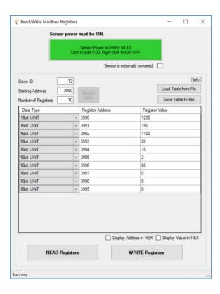
Both 16-bit (default) and 32-bit register sizes are supported. Whenever Modbus registers are read, the register size is changed to match the incoming data. The Data Type pull-down only lists data types that support the register size and unsupported data types in the register list are changed to the default data type for the register size.
