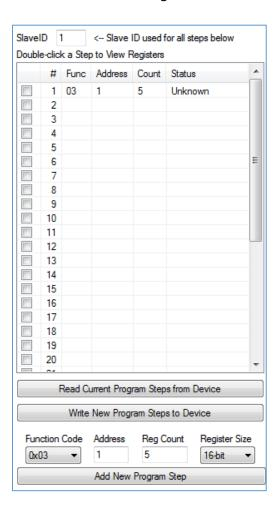
*Note*: In the legacy menu, the Register Addressing Mode is locked to One Based Addressing, so 3990 should be entered as 3991.
