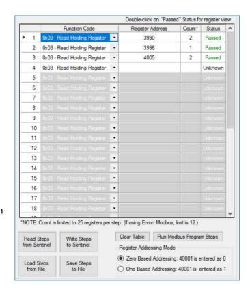
Click **Read Steps from Sentinel** to view the current program steps in the table. To add a new program step, fill in the next empty line. To delete a step, click on the line number and press the Delete key. Lines can also be copy/cut and pasted. Once all the desired program steps have been entered, click **Write Steps to Sentinel** to save the changes.
