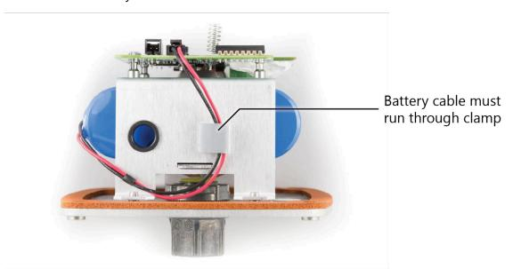
Plug the internal lithium battery pack into the connector labeled LITHIUM BATTERY as show below. Be careful to insert the battery connector as pictured with the locking tab facing up.
