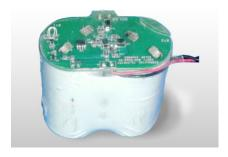
Solar Battery Power IQ Smart -Battery Pack For use with the A2 and HART modules
